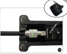
Place spacer 4 into the compression frame. Make sure the connector and cable both lay flat in the compression frame.
