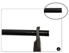
Straighten cable. Cut off the cable head.
