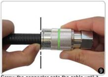
Screw the connector onto the cable until it reaches the marked line. Over tighten is forbidden.
