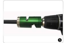
Insert the cable into the trimming tool. Select the low speed on the drill or 400~600 RPM on a variable speed drill. Trim the cable until no further debris generated.
